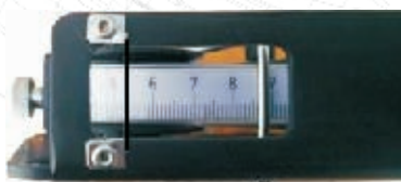
Level reading on graduated tape
