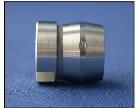
PIT ON SPECIMEN AFTER TEST
