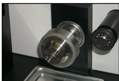
CLOSE-UP OF TEST RING IN-SITU
