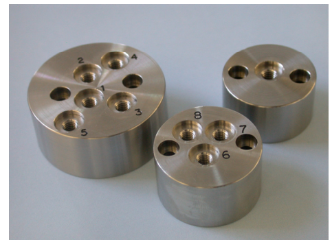
STROKE LENGTH SELECTOR FOR THE RECIPROCATING OPTION
