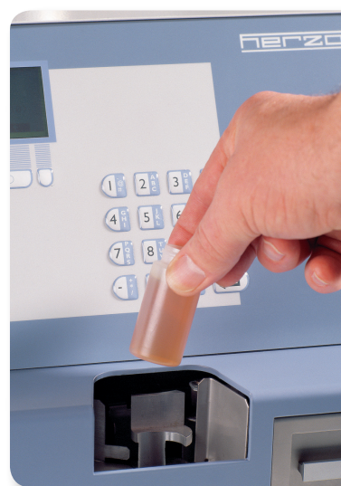
1. Insert sample beaker into feeder
