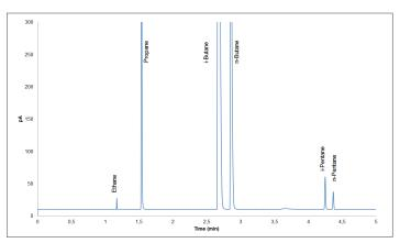
LPG Sample Analysis using the Hi-Speed RGA
