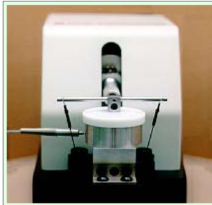
Above - The upper and lower specimen holder with PTFE seal
