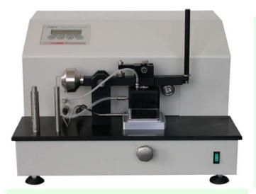
To determine the scuffing resistance of a fuel, a number of tests are carried out on the fluid sample using a stepwise series of loads. The load sequence is followed until the maximum load which can be applied without causing scuffing has been determined. The higher the SL-BOCLE load rating a fuel has, the more resistant it is to scuffing.
