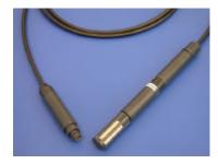
The ambient temperature and humidity is recorded using the HFRR integrated humidity probe. A humidity checker is available from PCS.
