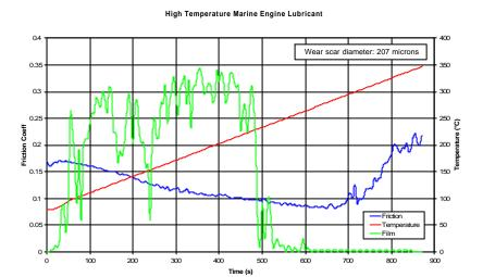
In diesel fuel test configuration the HFRR is fitted with low power heaters for maximum safety which can perform tests at up to 150°C. For testing specialised lubricants we offer a very high power heater option which allows tests at temperatures up to 400°C.
