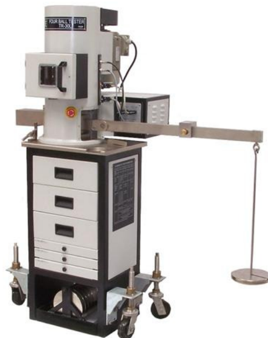
Ducom—TR 30 L machine with dead weight loading
