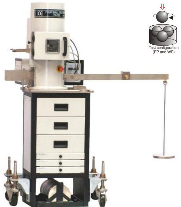
Ducom—TR 30 L machine with dead weight loading
