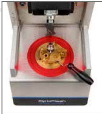
Optical fire detecting system covers entire hot area
