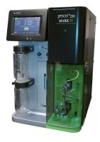
Put the IHT with the JFTOT results into the OptiReader
